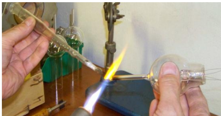
30 Melting the female taper joint to the tube
