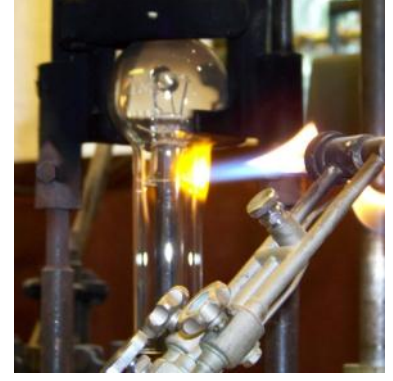
16 heating up the glass with a gas burner
