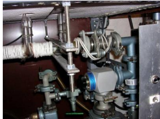
25 Vacuum rack connected to the diffusion pump
