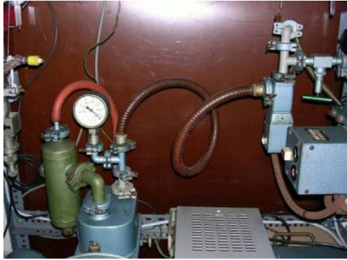
26 Connection of rotating pump and diffusion pump
