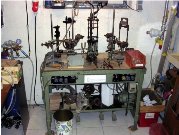
1 Gladitz glassblower vertical turning lathe
