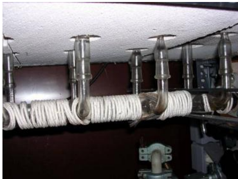
27 Vacuum rack with glass joints
